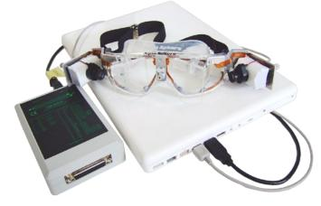
The EyeSeeCam VOG system is a full featured binocular 3D Video Occulo-Graphy system with a high spatial and temporal resolution. The lightweight system is designed to be totally mobile and remote controlled via Wireless LAN. You can connect external analog and digital signals to synchronize and capture additional experimental data. A 6 DOF inertial measurement unit is included by default. A database system enables you to organize your VOG experiments.
