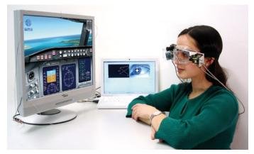
In combination with infrared LEDs or a pair of external stereo cameras it is possible to calculate the intersection of the user's gaze with any flat surface, i.e. a computer screen or a desk, while moving the head freely.
